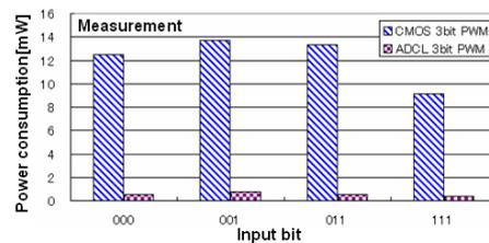
Fig. 7. Comparison of power consumption
