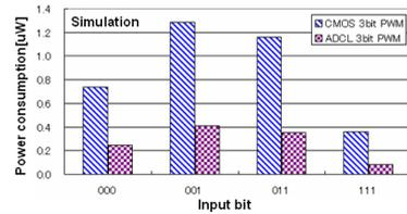
Fig. 4. Comparison of power consumption
