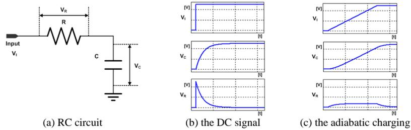
Fig. 1. Operation of a RC circuit
