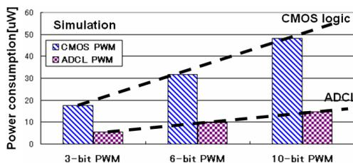
Fig. 8. Comparison of power consumption
